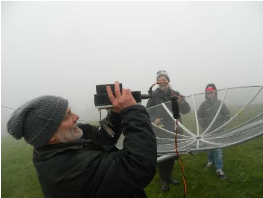
The 23cm-parabola has been put together – a last checkup onto the preamp and PA. In the background you can see Natthias, DM5CT and Max, DN2MAX
