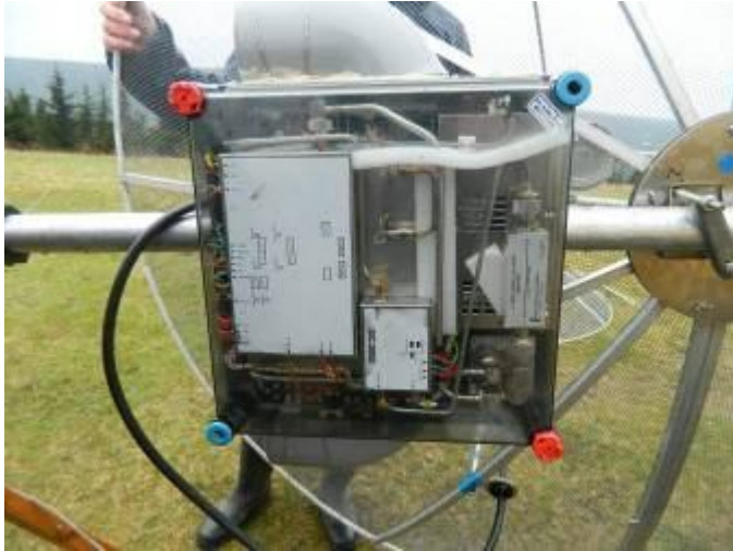
The 23 cm-PA is put together including its telemetry - upchecked by Harti, DL6AUI
