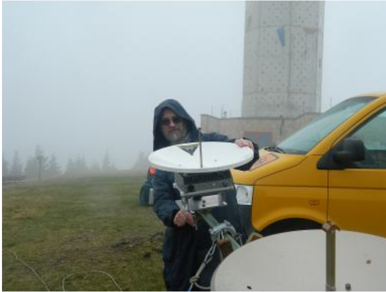
Matthias, DM5CT checking the direction of the 6 cm, 3 cm and 1,2 cm parabolas
